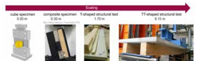
Fig. 3: Methodical approach for experimental test specimens from small laboratory specimens through to specimens at full component scale. © Fraunhofer WKI, Univ. Kassel FBH, TU Braunschweig ifs
