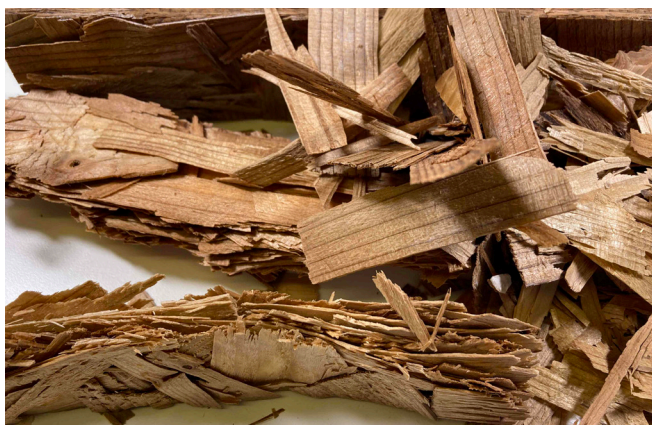
Fig. 3: OSB flakes with more or less dissolved Recyclamine adhesive, which releases the individual OSB flakes for reuse. © Peter Meinschmidt
