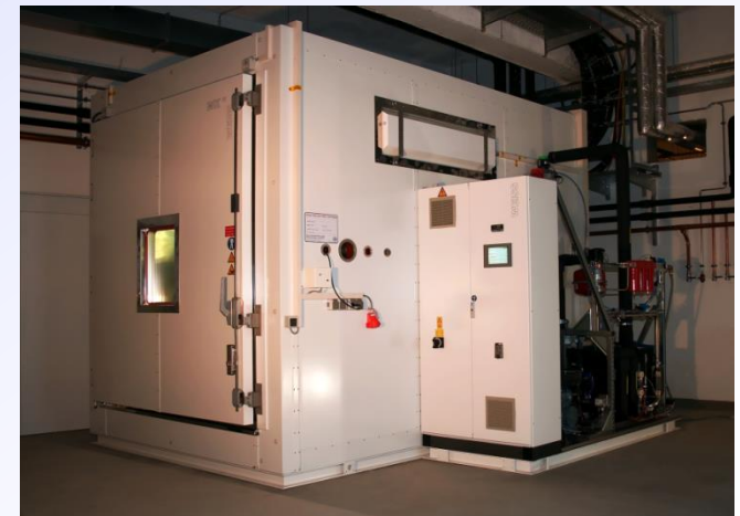
24 m 3 stainless steel chamber
